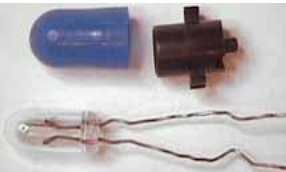
4. Remove old bulb from plastic holder
