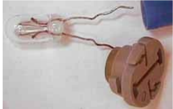
4. Separated bulb from plastic holder
