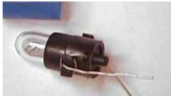
7. Loop wire into center notch of plastic
