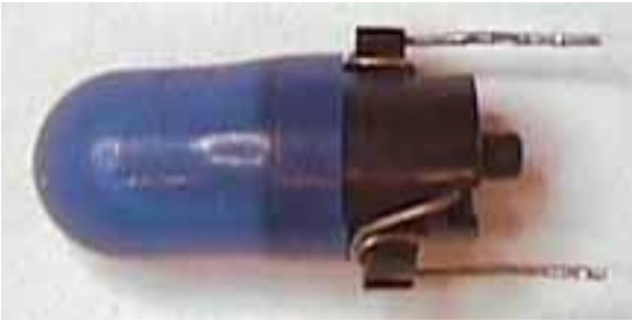
1. Remove bulb from the PCB
