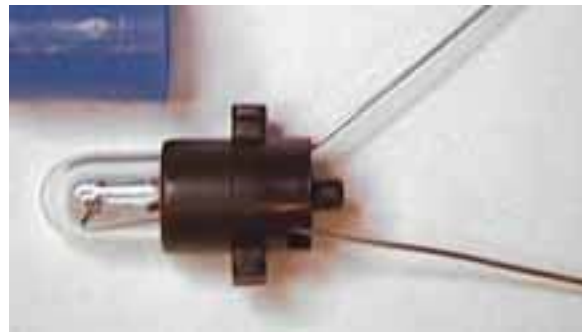
6. Insert new bulb into plastic holder
