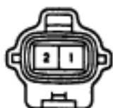
A30 ABS Speed Sensor Rear LH
