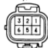
Door open Detection Switch (in Door Lock Assembly)
