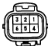
Door Courtesy Switch (in Door Lock Assembly)
