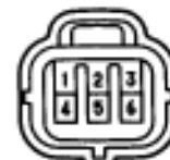
E1 No. 2 Solenoid Valve for ECT
