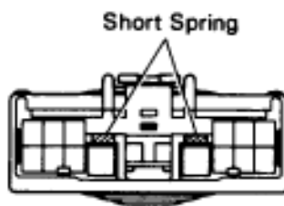
Center Airbag Sensor Assembly Connector (Connector ①)
