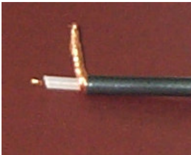
Figure 7: Stripped back sheath and twisted braid
