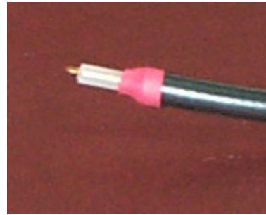
Figure 6: Stripped back sheath and insulated braid
